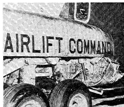
Fig. 6 C-141 main landing gear fairing damage.
